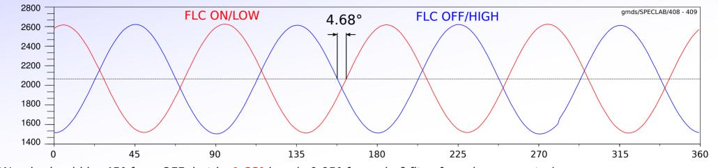
ON axis should be 45° from OFF, but is **4.68**° less ( $\pm 0.05^{\circ}$  from *sin*  $\theta$  fits of avg image centre). This is apparently fairly temperature sensitive.
