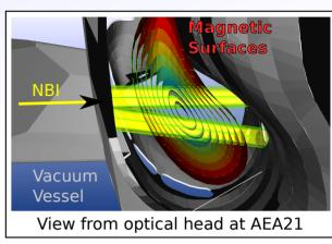
MSE is difficult in stellarators because pitch angle and Doppler shift vary across the beam width, making a very complex polarised spectrum.
