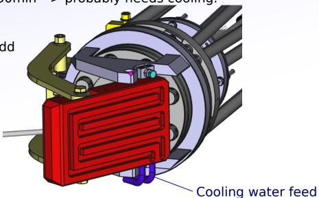
2) Some kind of flexible thermal conductive strip to cooled block
