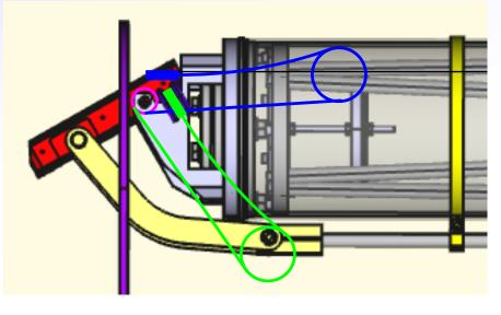
Two coils of pipe required to deal with offset as well as rotation.
