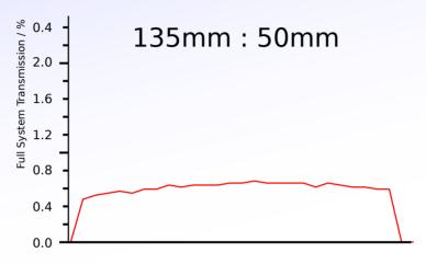
Some proportion of the light goes through the filter at a very steep angle and shifts the filter short-pass into the useful spectrum. The filter functions for different image positions calculated by the ray tracer are shown below. These assume a filter effective index of n = 2.0 and an ideal sharp 655nm short-pass filter at normal incidence:
