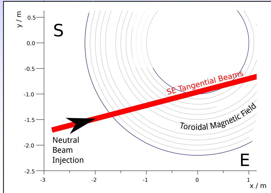
Neutral beam atoms injected into plasma.
