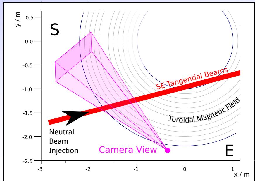
Neutral beam atoms injected into plasma.
