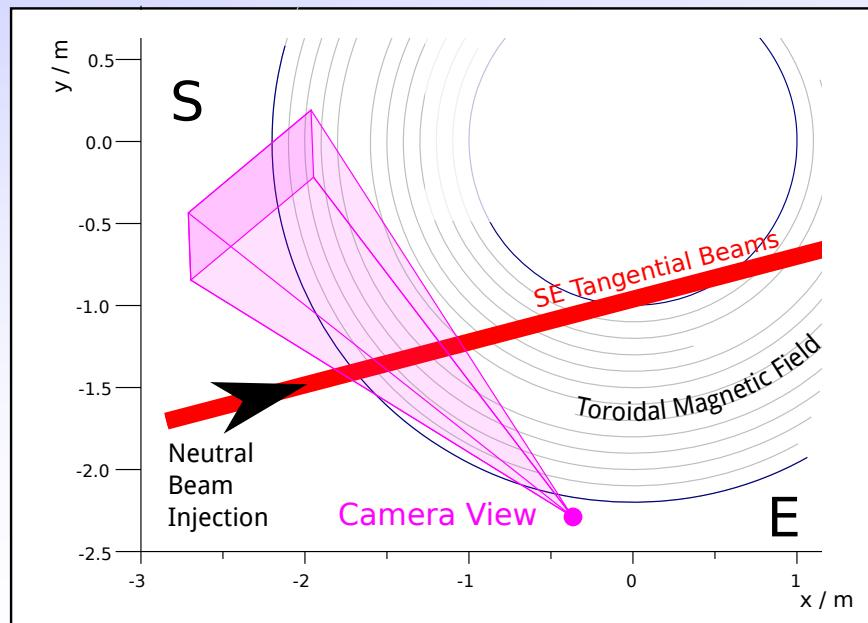
Neutral beam atoms injected into plasma.
