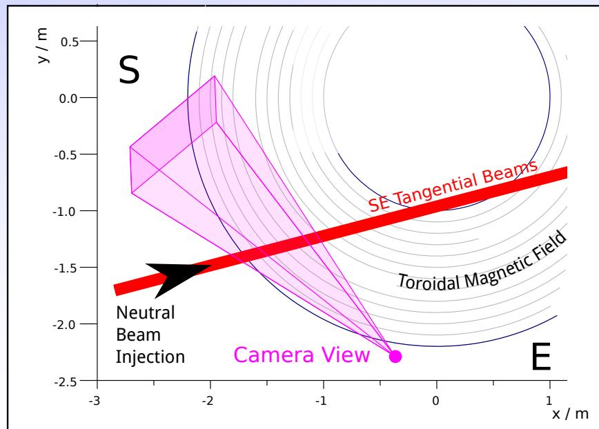
Neutral beam atoms injected into plasma.
