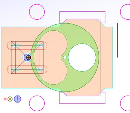
Position sensor using PC Mouse. Was less accurate than trusting the stepper motor, so removed.
