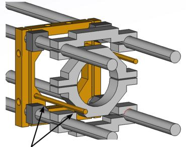
Locator rods need to avoid positioning stubs and fibre clamp
