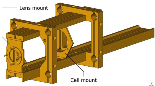
2) Add top and bottom rails that keep carriage stiff and allow optical element mounts to slide along:
