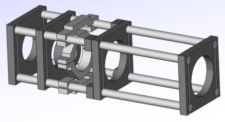
2) Build the IMSE system (at HGW) as a complete unit which slides on to the 4 rails. It must avoid the positioning stubs and the fibre holder clamp:
