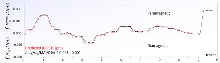
i.e: Variation of integrated toroidal field matches calculation from poloidal field, GS equ and CLISTE's assumptions. We can very probably trust that the integral is really diamagnetic.
