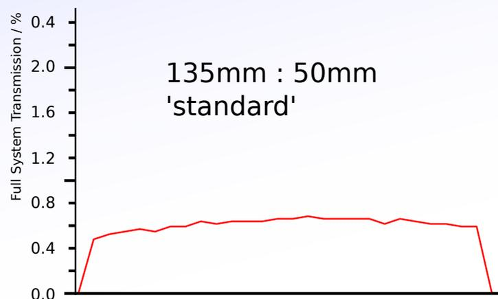
Some proportion of the light goes through the filter at a very steep angle and shifts the filter short-pass into the useful spectrum. The filter functions for different image positions calculated by the ray tracer are shown below.
