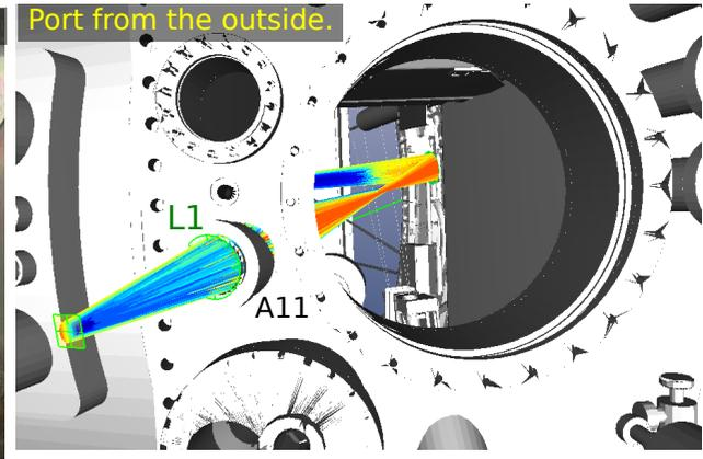
Option 1: Focusing mirror (ellipsoidal):
