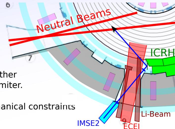
Optimising the optical system within the IMSE forward model, bounded by the mechanical constraints leads to a more compact system than the standard MSE.
