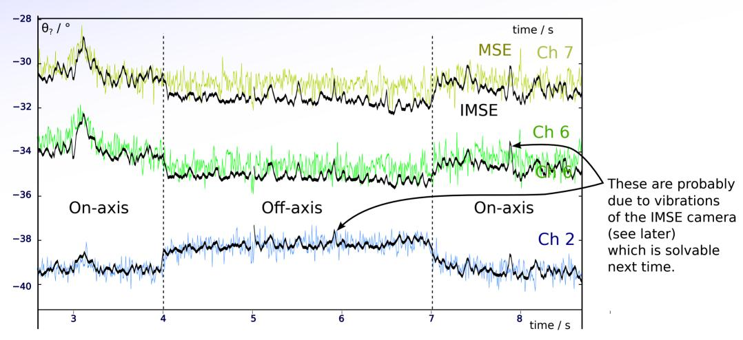
This gave me some concern that the IMSE is susceptible to background contamination. Here, the background drops by  $\sim\!20\%$  during the off-axis period (probably changing charge exchange H $\alpha$  'Halo' or FIDA emission).
