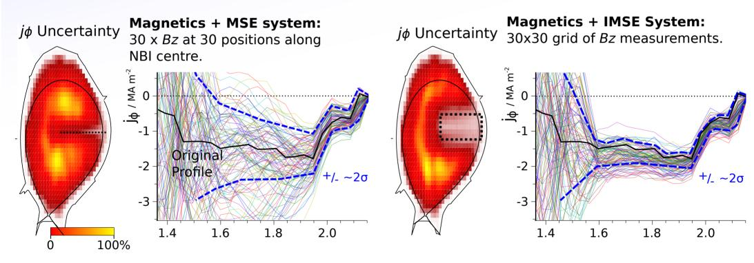
Each case has 900 measurements at  $\sigma = 10mT$ . So difference is only in the **type** of information.
