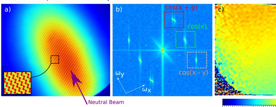
The polarisation angle relates directly to magnetic field pitch angle.
