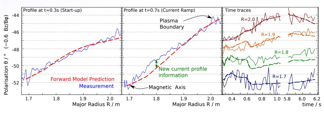
At present, the diagnostic has **no angle calibration**. The forward model is based entirely on the CAD and optics models and the measurement is unprocessed.
