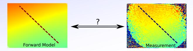
Compared directly with the measurement, there is only a 0.7° offset. Once subtracted, it agrees during current ramp with the regions where the equilibrium/CT is expected to correctly predict the pitch angle:
