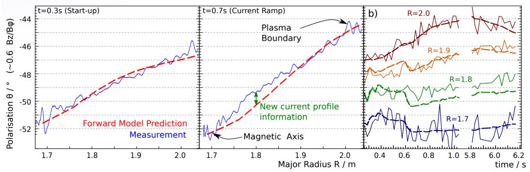
At present, the diagnostic has **no angle calibration**. The forward model is based entirely on the CAD and optics models and the measurement is unprocessed.
