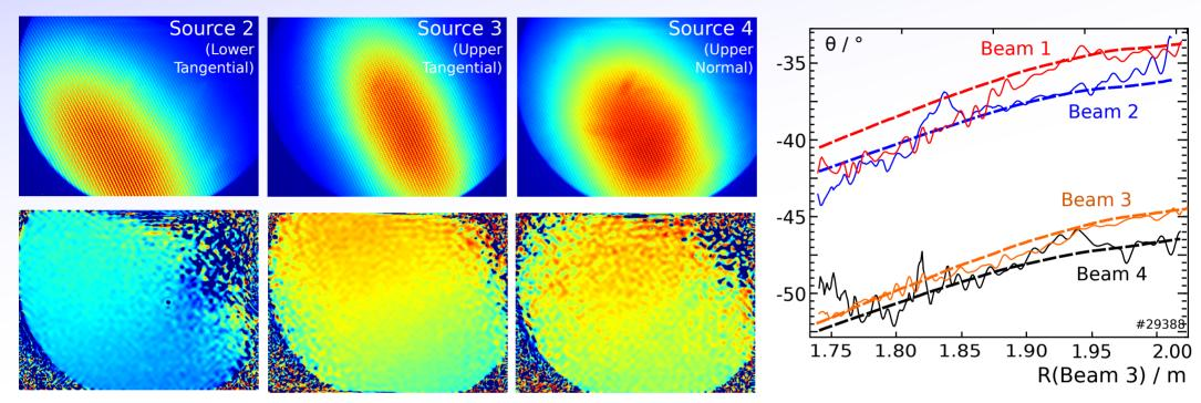
$\theta_3 - \theta_1$  is a fixed geometry value, so the agreement confirms the diagnostic linearity and beam geometry.  $\theta_3 - \theta_4$  (or  $\theta_2 - \theta_1$ ) relate directly to Bz/B $\phi$  and are unaffectd by fixed offset errors.
