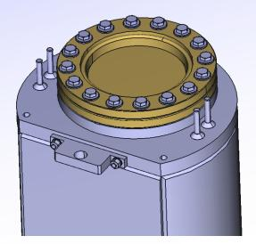
Pfeiffer Vacuum standard CF100 Fused Silica vacuum window UHV compatible. Max 200'C.
