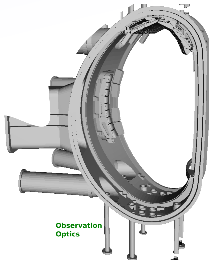
ASDEX Upgrade Vacuum Vessel
